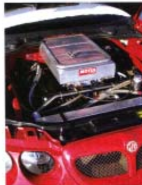
Above: 765bhp version of Ford V8 was to be offered in the MG SV.
